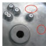
Compression Mold Defect Detection
