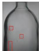
Surface Defect Detection of Transparent Bottle
