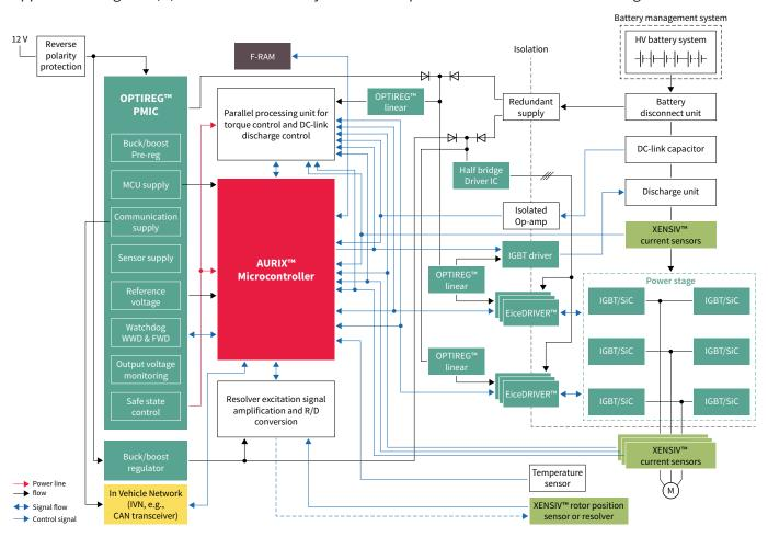
Application diagram: (H)EV traction inverter system with in-phase and DC-Link current sensing
