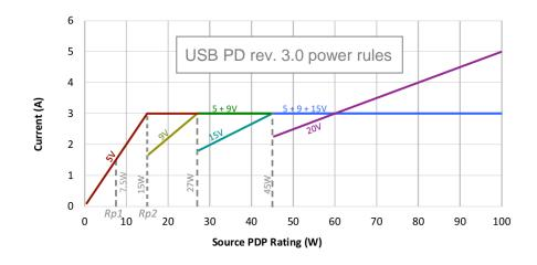
Most power levels for single automotive USB ports: 15-27W
