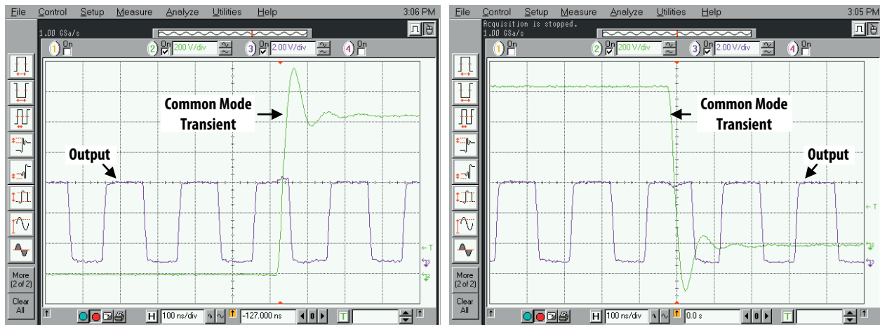
Figure 13. High voltage common mode noise spike hardly causes a ripple in the output of 10MBd digital optocoupler ACPL-M61L.
