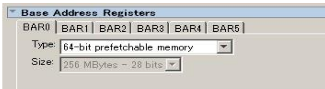
図 2-6. PCI Base Address Registers
